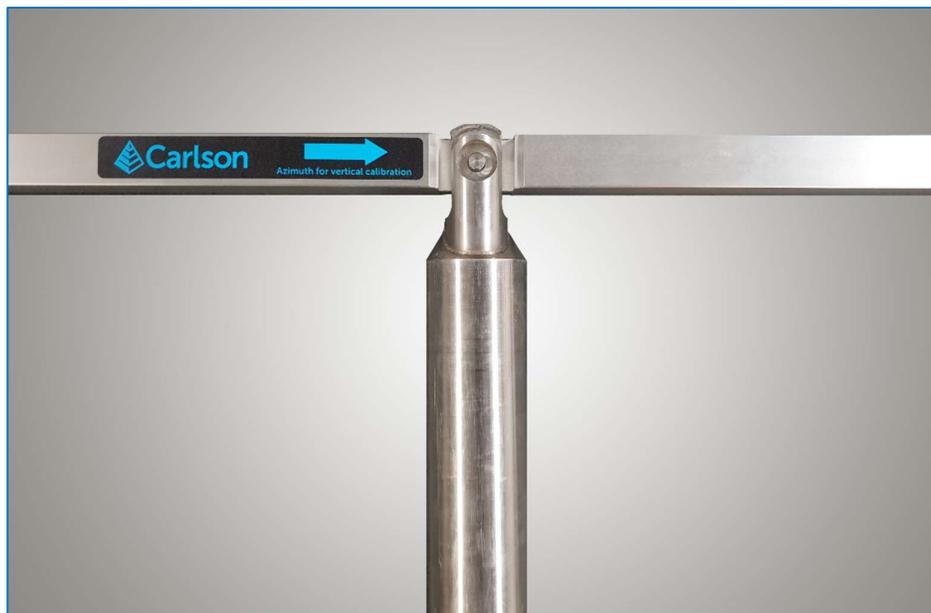
*Figure 35 C-ALS hanging from adaptor for vertical alignment*
