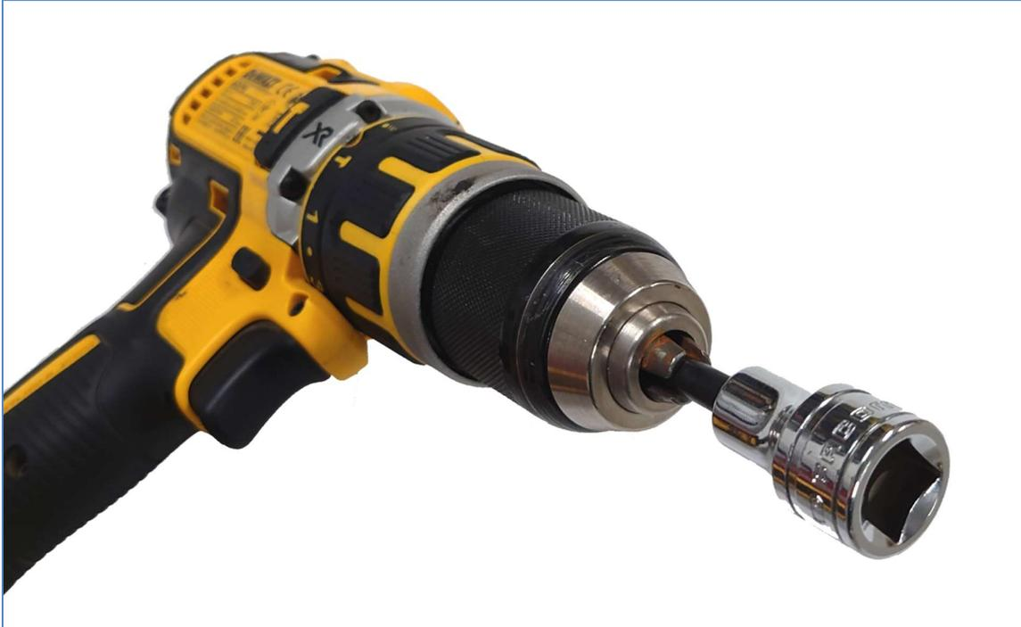
*Figure 19 Drill with 1/4" socket attachment*
