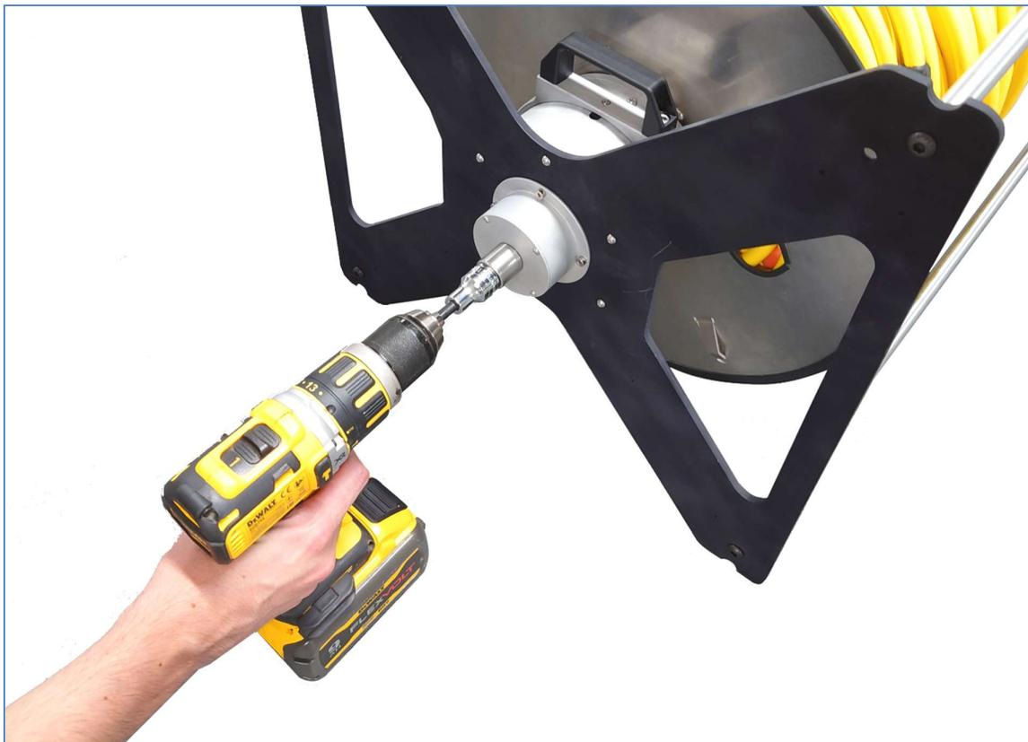
*Figure 20 Using a drill to operate the winch*
