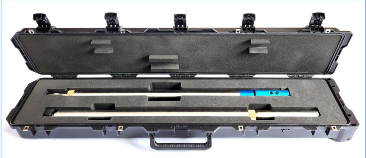
*Figure 29 C-ALS probe and extension piece in their transit case*
